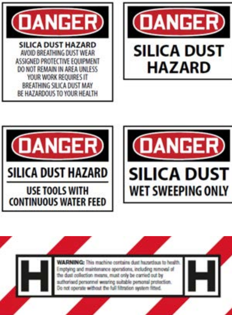
Figure 6 Examples of dust hazard signs
