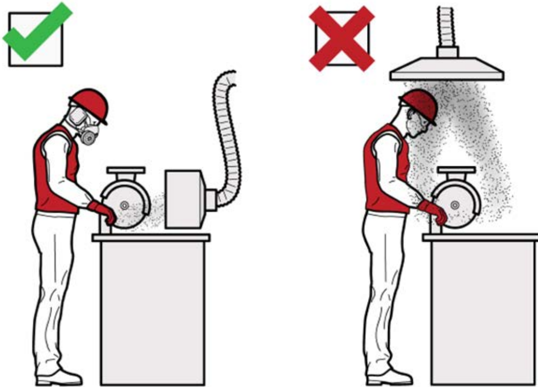
Figure 5 Examples of using local exhaust ventilation
